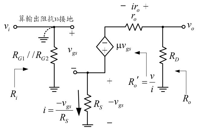
$$A_v = \frac{v_o}{v_i} = \frac{-\mu v_{gs} \times \frac{R_D}{R_S + R_D + r_o}}{v_{gs} + \mu v_{gs} \times \frac{R_S}{R_S + R_D + r_o}} = \frac{-\mu R_D}{1 + \frac{\mu R_S}{R_S + R_D + r_o}} = \frac{-\mu R_D}{r_o + R_D + (1+\mu)R_S}$$
