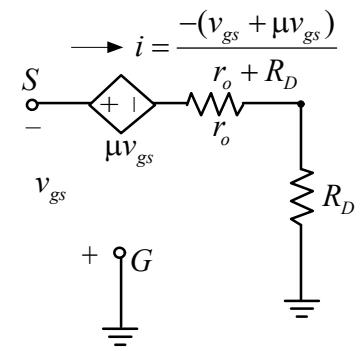
$$R_i = R_S // R'_i = R_S // \frac{v}{i} = R_S // \left( \frac{-v_{gs}}{\frac{-(1+\mu)v_{gs}}{r_o + R_D}} \right) = R_S // \left( \frac{r_o + R_D}{1 + \mu} \right)$$
